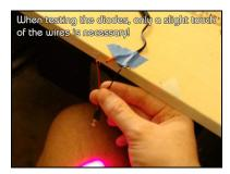
I just taped the wires from the power supply in a fixed position and all I do is barely touch the appropriate wires together. If it lights up... congrats! That diode works! Literally, I could test one diode probably every five seconds or less so this didn't take long at all!
